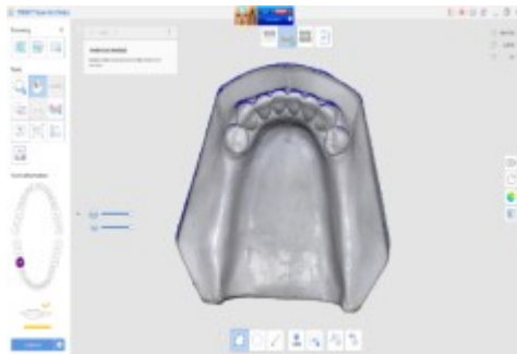
Figure 3: Optically scanning of the epoxy cast
