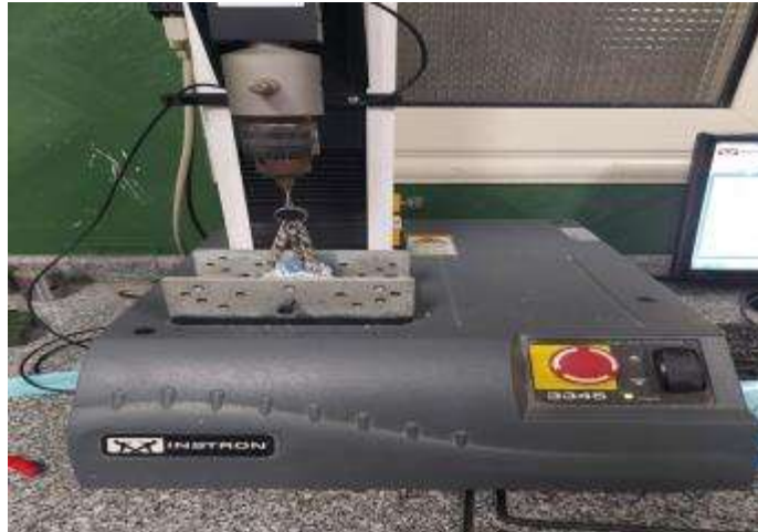
Figure 9: Instron pull out the framework centrally
