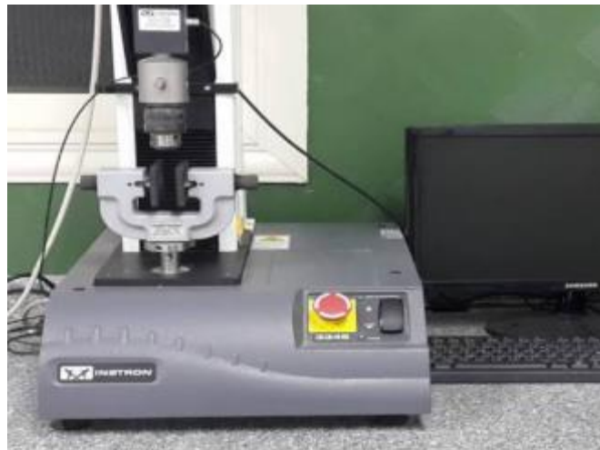
Figure 8: Instron model 3345 universal testing machine
