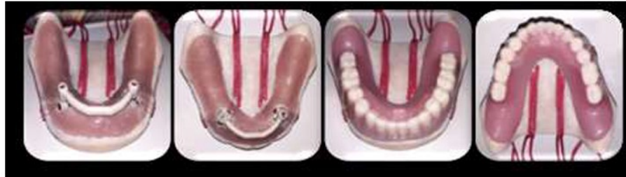
Figure 4: view after installations of strain gauge rosettes
