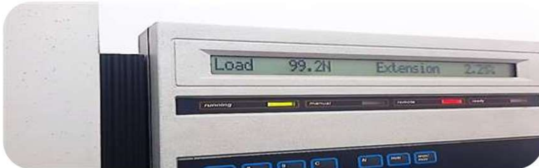
Figure 6: View showing screen load of the universal testing machine during the test.
