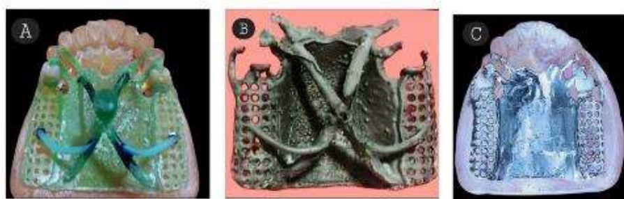
Fig.5 A: spruing of printed resin RPD framework. .B, 3D printed resin casted Frameworks after casting. c, the casted framework finished and fatted on the epoxy resin cast.
