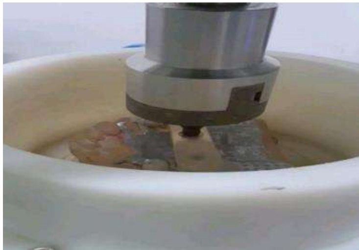
Fig.8 spherical tip of the chewing simulator applied a load on the RPD framework.
