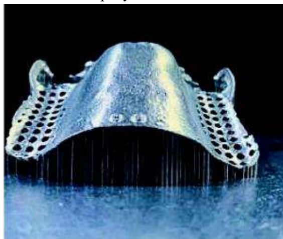
Fig.5 A: spruing of printed resin RPD framework. .B, 3D printed resin casted Frameworks after casting. c, the casted framework finished and fatted on the epoxy resin cast.
